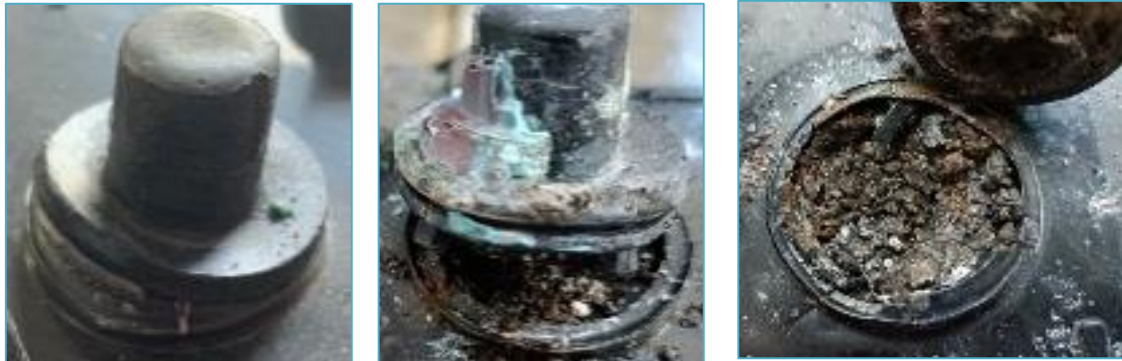
Positive terminal got deformed or corroded
